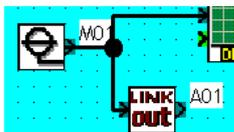
Link Function A01 needs to be activated to switch the GSM Modem ON. This can be done by triggering the block with an "Always On" contact.
