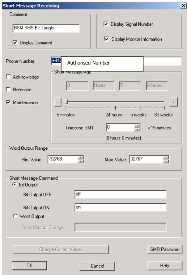
The above example allows bit output control based on incoming messages from the authorised mobile number shown in the "phone number" box only. It can also be password protected.
