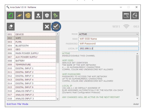
3. **PLMN** – This is the mobile network for the SIM you are using – Make ACTIVE then enter the mobile number of the SIM card in international format and the APN, username and password required for the network to make a data connection. If you are unsure of these just Google the network and APN.
