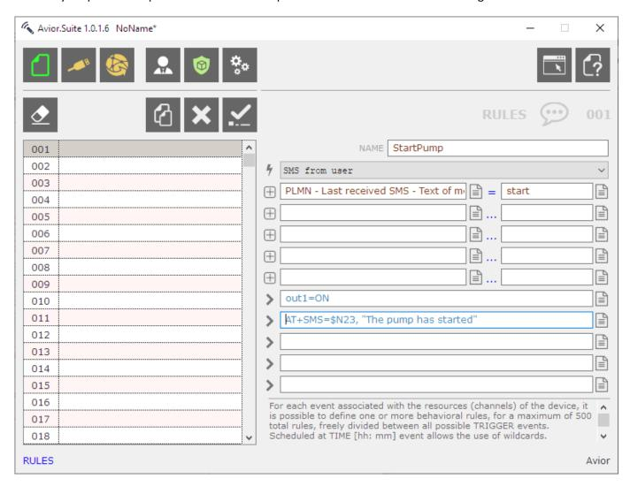
**RULES** – Rules consist of a TRIGGER (eg SMS from USER) and can be combined with up to 5 CONDITIONS (eg Last SMS received contains the word "start") and a subsequent ACTION (eg Turn Output 1 ON and send a SMS to the last sender \$N23) – up to 5 ACTIONS can be triggered per RULE.
