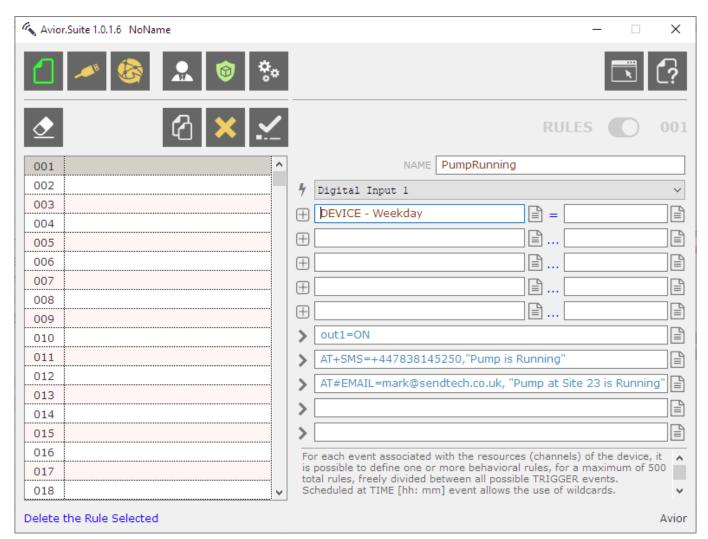
In this example when the triggers INPUT 1 is closed AND it's a WEEKDAY then action the commands to turn on OUTPUT1 AND send an SMS AND an EMAIL to confirm the pump is running (all in the one RULE).
